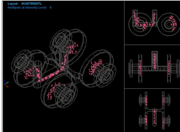
Figure: 6 Major hotspot at intensity level 9 in initial gating design.
